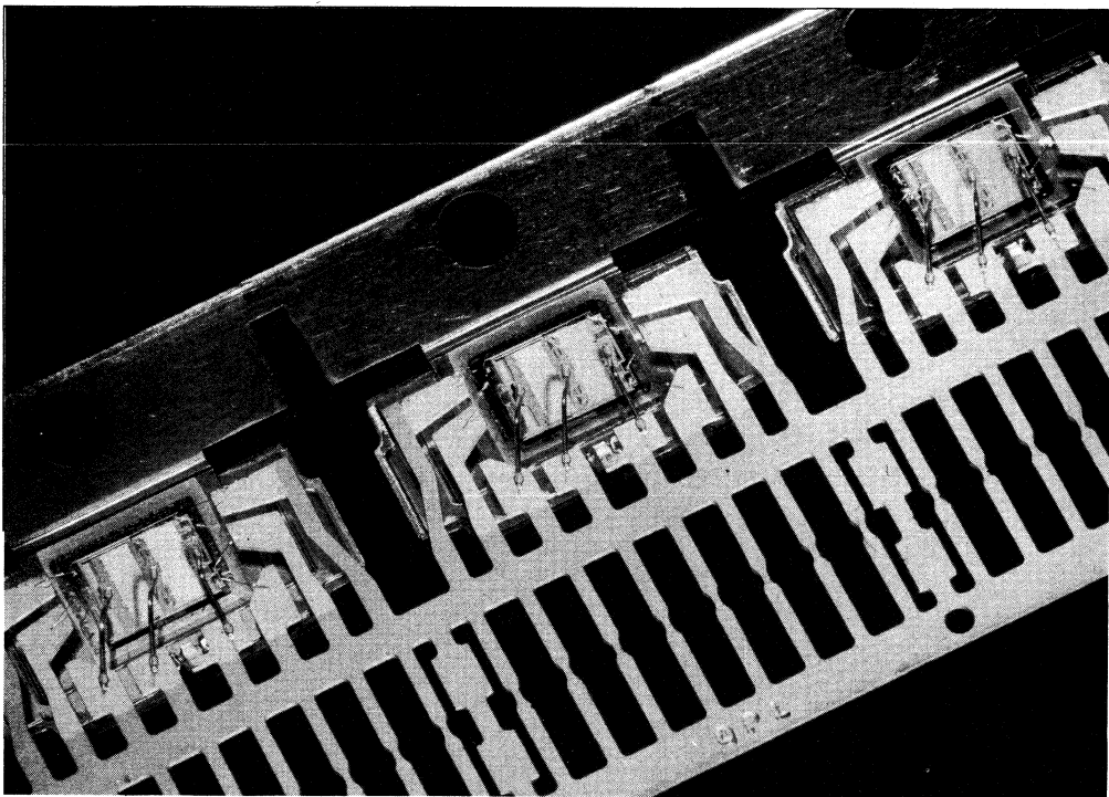
Figure 9: An example of a power IC using mixed wire bonding.
